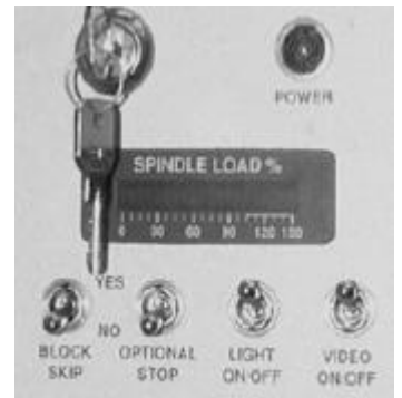
Figure 2-3 KEY LOCK used to protect unauthorized editing of programs.
